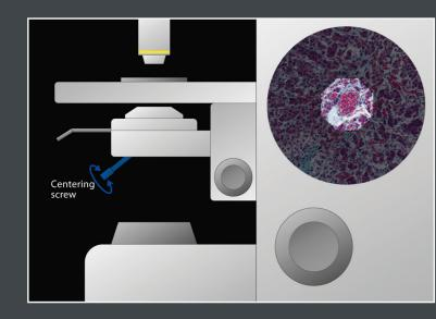
5.00 Center the luminous field stop image with the condenser centering screws.
