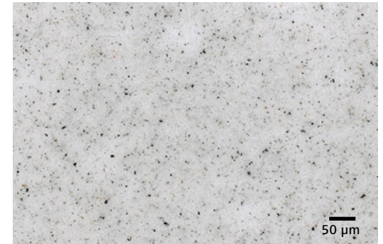
Particle analysis, brightfield, objective: EC Epiplan-NEOFLUAR 20×/0.5
