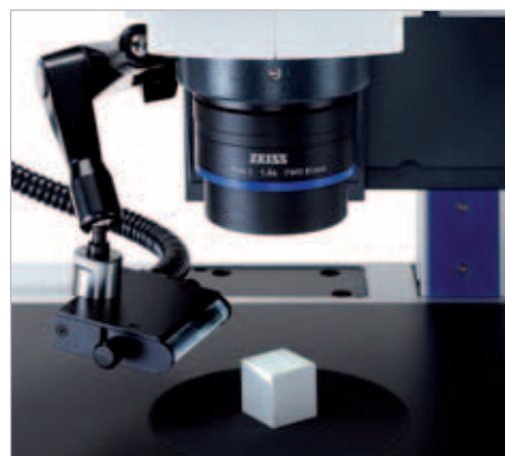
Line light S, l=50\text{ mm} Turns the light guide's circular cross section into a narrow fiber-optic slit. The light, which is projected at an extremely flat illumination angle, strikes the top of the specimen at a flat angle, and the corresponding shadow effect makes even the smallest surface structures become visible. Also well-suited for use with objectives with short working distances.
