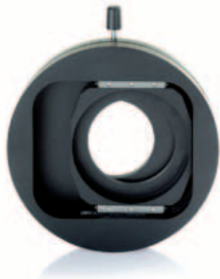
Objective slider S/doc Designed to switch the objective between: ■ The stereoscopic observation position ■ The axial mode position, providing a parallax-free view of the specimen through the stereo microscope's left or right (figure above) observation channel
