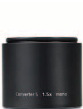
Converter S 1.5x ■ The Converter S 1.5x increases the magnification and resolution levels in axial mode (tandem mono combination) by a factor of 1.5. ■ The objective's free working distance, on the other hand, stays the same.
