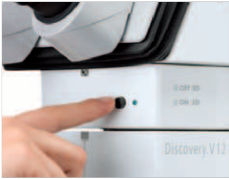
When you use axial mode to observe an object through the binocular eyepiece tubes, you first need to move the objective by pushing a button to center it underneath the stereo microscope's right-hand channel. The activated beam-splitter configuration then allows you to observe the microscopic image in 2-D and without any parallax.
