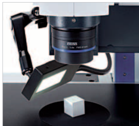
Diffuse facelight M8 Indirect, soft oblique illumination prevents outshining reflections
