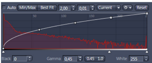
As seen here, a nonlinear Gamma curvature in the range of 0.45 over the whole dynamic range often delivers good results for transmitted light images.
