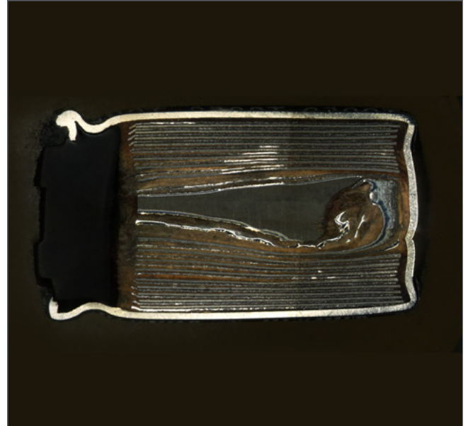
Foil capacitor, cut open, with dielectric in between; acquired with ZEISS Axio Zoom.V16, reproduction of object/camera 0.8
