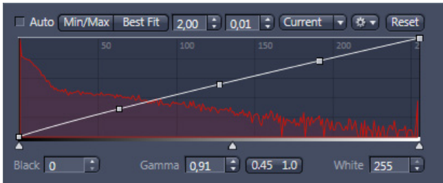
A nearly linear Gamma over the whole dynamic range delivers a rather dark display of this transmitted light image.
